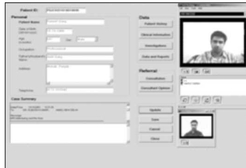
► Fig. 12.7 Integrated display of data and video images in videoconferencing setup for telemedicine
