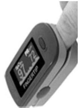
► Fig. 9.10 Finger tip complete Pulse oximeter (Courtesy: FaCT Canada Consulting Limited)
