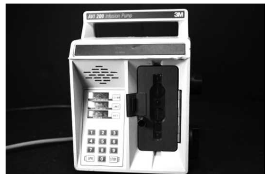
► Fig. 35.8 Programmable microprocessor based infusion pump (Courtesy: AVI, Inc. U.S.A.)
