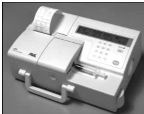
► Fig. 15.18 Critical care analyser for measuring blood gases and other parameters (Courtesy: M/s AVL Medical Instruments)
