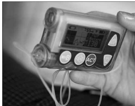
► Fig. 35.13 Typical insulin pump (Courtesy: M/s Medtronic, U.S.A.)
