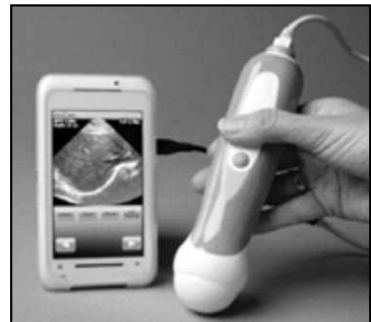
▶ Fig. 23.36 A portable mobile phone and ultrasound scanning system (Courtesy: Mobisante, U.S.A.)
