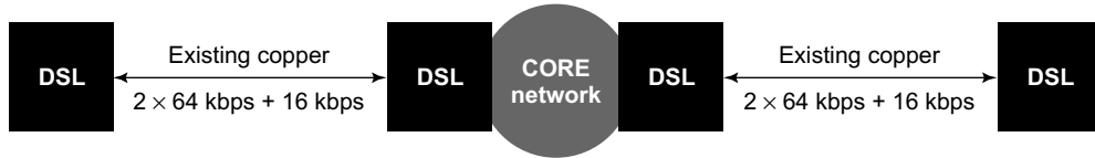
► Fig. 12.9 Principle of use of digital subscriber line (DSL) modem for computer communication
