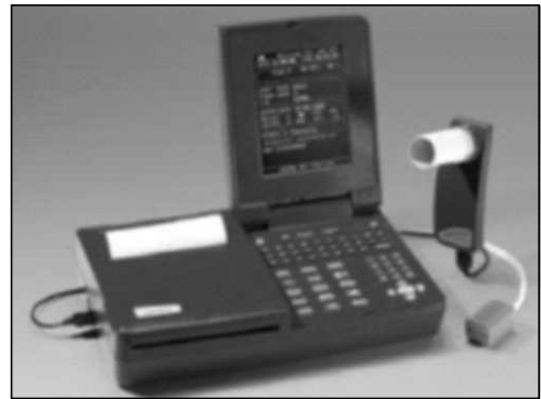
► Fig. 13.9 Desktop spirometer (Courtesy: M/s Smiths Medical)
