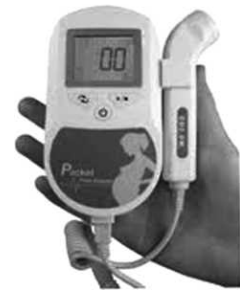
► Fig. 8.8 A typical ultrasonic blood flow detector
