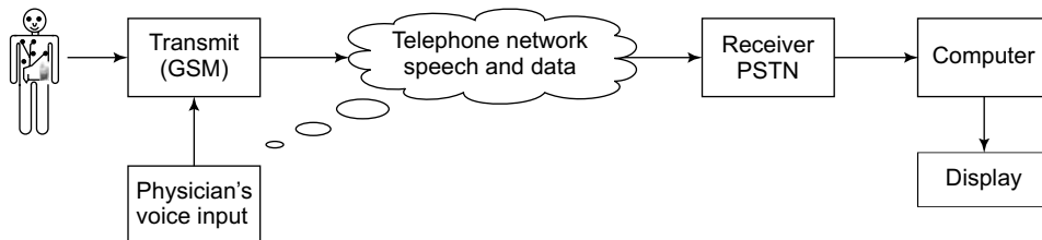
► Fig. 12.24 Telecardiology system based on cellular telephone communication, wherein speech and data are carried simultaneously over a single GSM channel (Scanlon, 2000)
