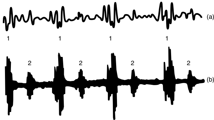
► Fig. 8.4 Foetal phonocardiogram: (a) unfiltered heart sound, (b) filtered heart sounds
