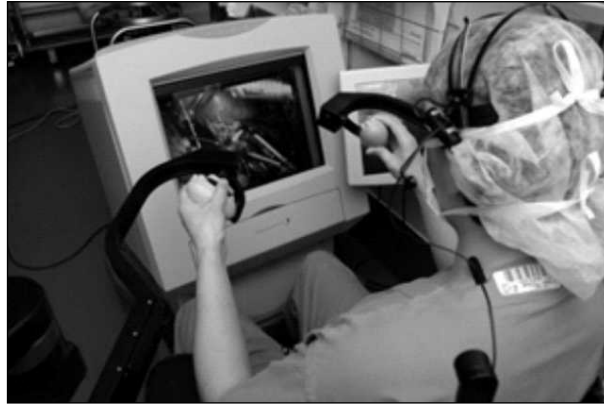
► Fig. 12.21 An urological surgical operation (telesurgery) being performed using three-armed ZEUS robot
