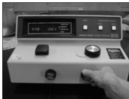
► Fig. 14.11 A single wavelength spectrophotometer
