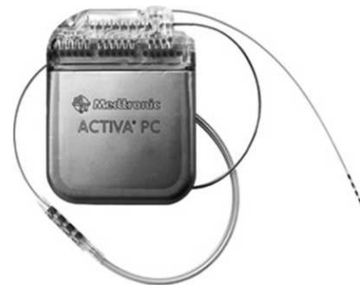
► Fig. 29.20 Neuro stimulator (Courtesy: M/s Medtronic)
